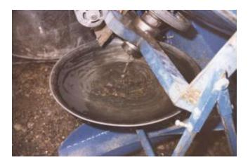
By the time this process was finished the gold pan would be primarily gold, with a very little bit of black sand.
